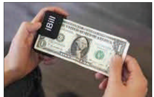
Photo: A person's hands holding an iBill Currency Reader situated at the top left-hand corner of a $1 bill.
