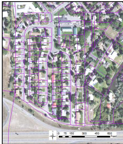
Figure 3: Example of existing cadastral shift in the City of Livingston, despite previous PLSS adjustments.
