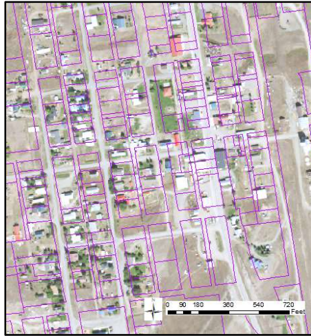
Figure 2: Example of existing cadastral shift in the community of Wilsall, despite previous PLSS adjustments.
